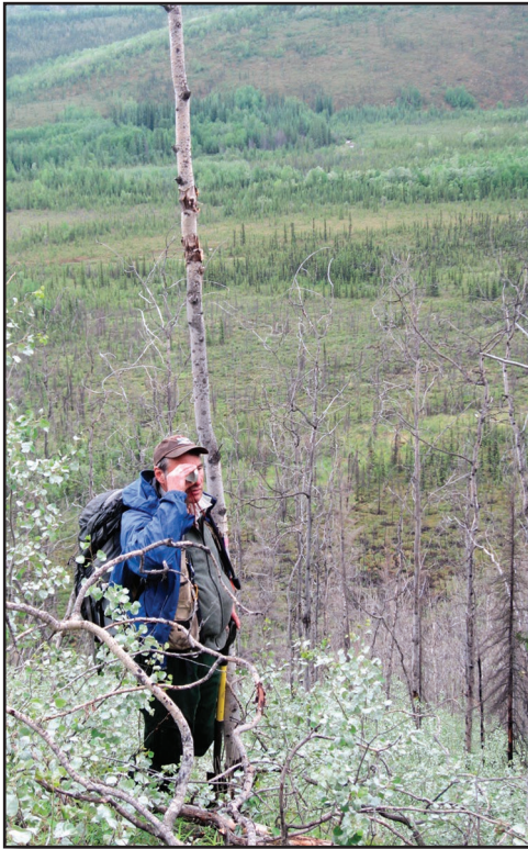
Figure 12–8—A clinometer is used during trail layout reconnaissance to measure sideslope (see table 12–4).
