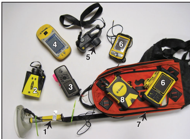
Figure 9–1—Examples of Global Positioning System (GPS) units and support hardware used for trail mapping work. Clockwise from bottom left: external GPS antenna (1), laser rangefinder (2), recreation-grade GPS receiver (3), mapping-grade GPS receiver (4), digital camera with integrated GPS and compass (5), data loggers (6), field GPS backpack (7), and mapping-grade GPS receiver (8).
