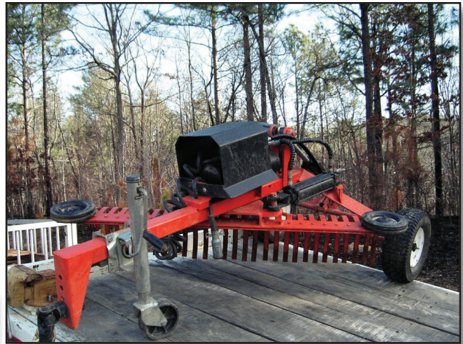
Figure 14–3—A spring-tooth rake is pulled by an all-terrain vehicle for final tread shaping.
